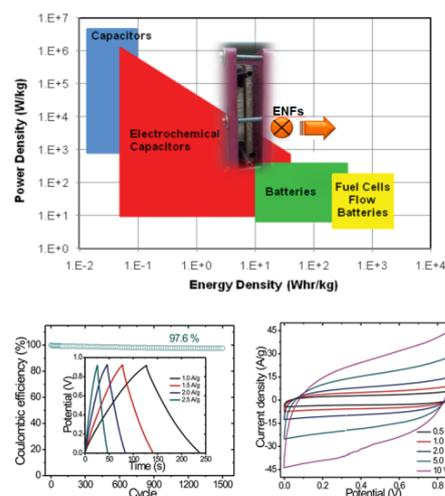
**Fig) Top:** Power and energy densities of various Electrochemical Energy Storage (EES) systems. The orange circle marks the performance of the electroactive nanofluid electrode for flow cells. Image of flow cell used for the charge-discharge measurements. **Bottom:** Charge-discharge curves at various current densities and excellent cyclability at least up to 1500 cycles.
