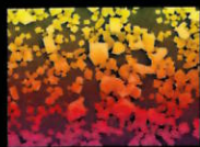
Submicron MOF crystals fabricated by spray-drying
